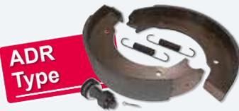
Replacement brake shoe kit for ADR type axle. 400mm x 80mm brake drum. One brake shoe kit per wheel is required. Kit includes springs and pivot bolt. Brakes should be checked every three months, being adjusted or replaced as necessary. It is recommended to fit brakes in axle sets.
